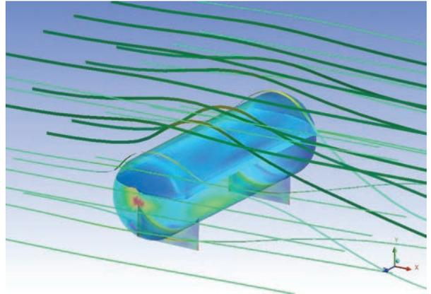
Time slice shows streamlines of explosion flow over pressure vessel.
